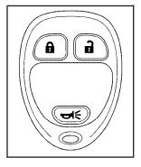
$\ensuremath{\widehat{\mbox{\rm c}}}$  (Lock): Press  $\ensuremath{\widehat{\mbox{\rm c}}}$  to lock all the doors, including the liftgate.
